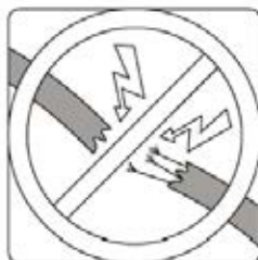
Check for damaged wires
